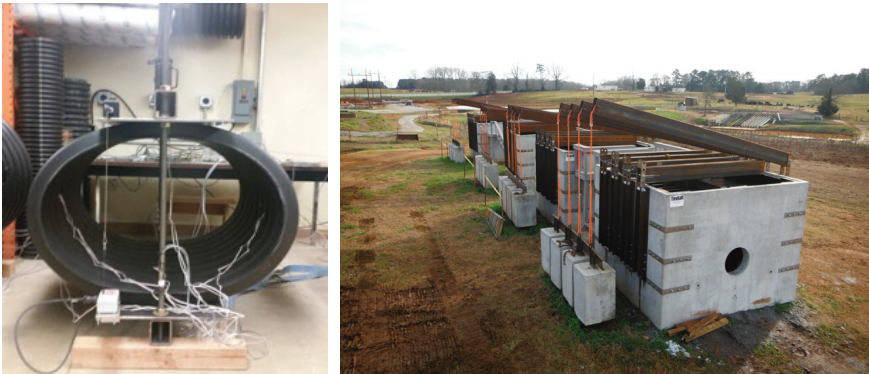
Figure 8.9: Laboratory and field testing on full scale pipes to validate the service life prediction model
